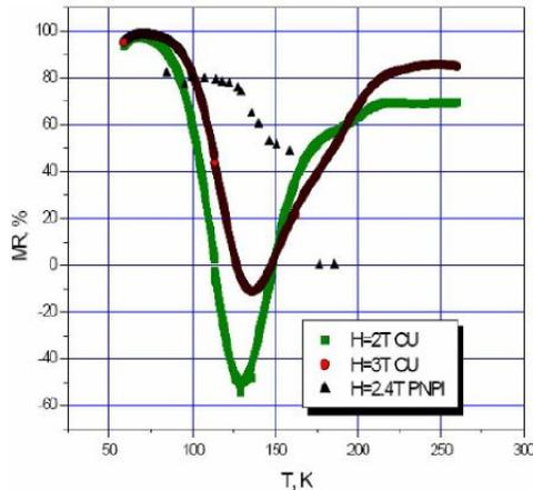
**Fig. 5.11** Magnetoresistance of  $Sm_{0.6}Sr_{0.4}MnO_3$  at different applied magnetic fields.
