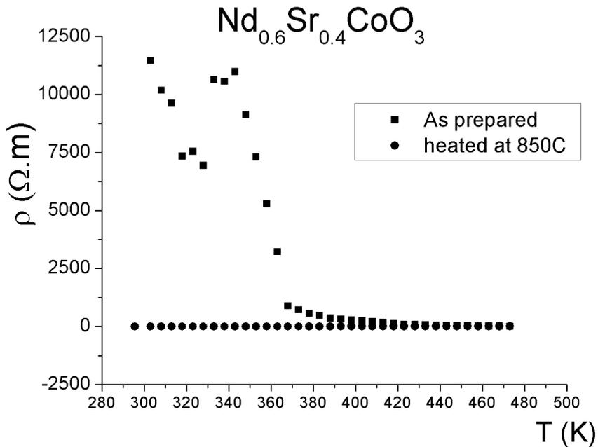
**Fig. 5.3** DC resistivity – temperature dependence of  $\text{Nd}_{0.6}\text{Sr}_{0.4}\text{CoO}_3$ .
