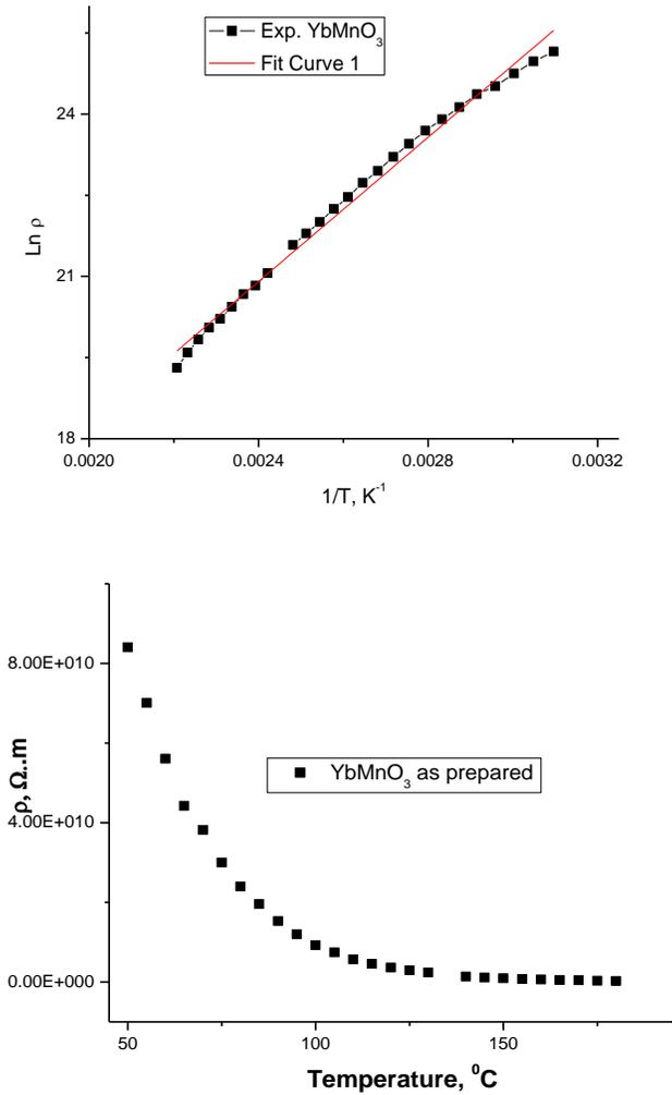
**Fig. 5.13** The DC resistivity – temperature dependence measurements of  $YbMnO_3$  as prepared.
