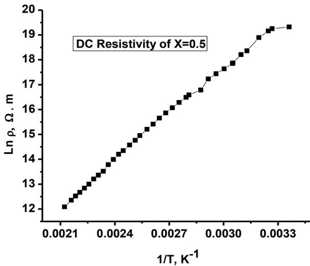
Fig. 5.2 DC resistivity – temperature dependence of  $\text{Eu}_{0.65}\text{Sr}_{0.35}\text{Fe}_{0.5}\text{Mn}_{0.5}\text{O}_3$ .
