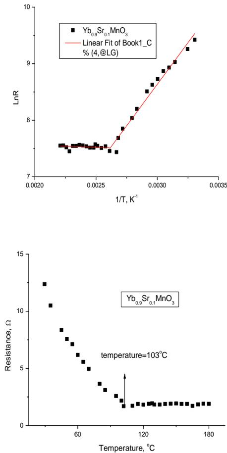
**Fig. 5.12** The DC resistivity – temperature dependence measurements of  $\text{Yb}_{0.9}\text{Sr}_{0.1}\text{MnO}_3$ .
