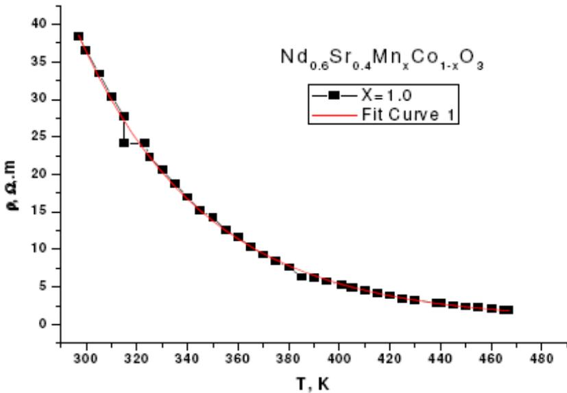
*Fig. 5.5 The DC resistivity – temperature dependence measurements of  $\text{Nd}_{0.6}\text{Sr}_{0.4}\text{Mn}_x\text{Co}_{1-x}\text{O}_3$  ( $x=1$ ).*
