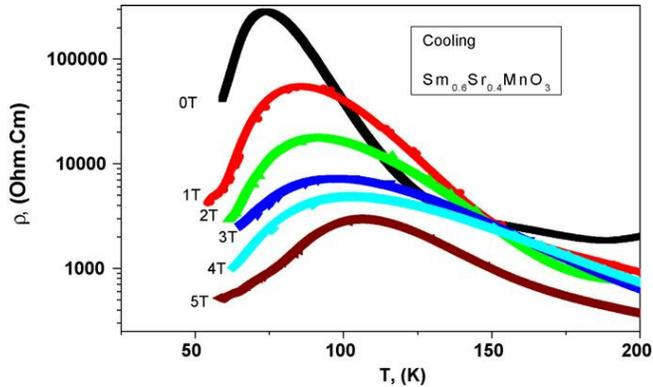
**Fig. 5.10** Thermal dependence of the resistivity at applied magnetic fields of 0 T, 1 T, 2 T, 3 T, 4 T and 5 T of  $\text{Sm}_{0.6}\text{Sr}_{0.4}\text{MnO}_3$  for cooling runs.
