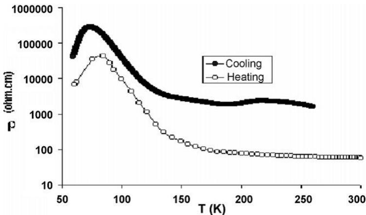
**Fig. 5.9** Temperature variation of resistivity at  $0\text{ T}$  magnetic field of  $\text{Sm}_{0.6}\text{Sr}_{0.4}\text{MnO}_3$  polycrystalline sample (in heating as well as in cooling).
