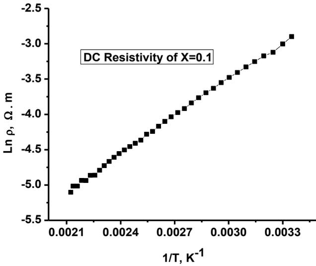
Fig. 5.1 DC resistivity – temperature dependence of  $\text{Eu}_{0.65}\text{Sr}_{0.35}\text{Mn}_{0.9}\text{Fe}_{0.1}\text{O}_3$ .
