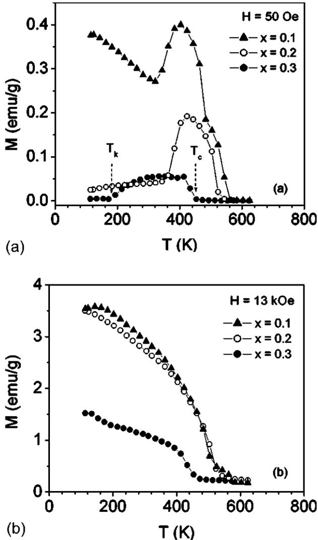
**Fig. 5.15** Temperature dependence of magnetization for the orthoferrites  $\text{SmFe}_{1-x}\text{Mn}_x\text{O}_3$  ( $x=0.1, 0.2, \text{ and } 0.3$ ) in the applied fields of (a) 50 Oe and (b) 13 kOe.
