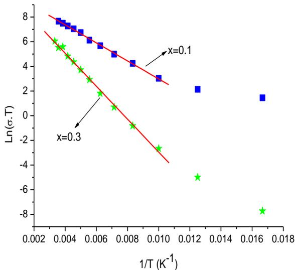
**Fig. 5.8** DC conductivity of  $\text{Nd}_{0.65}\text{Sr}_{0.35}\text{Fe}_x\text{Mn}_{1-x}\text{O}_3$  ( $x=0.1$  and  $0.3$ ).
