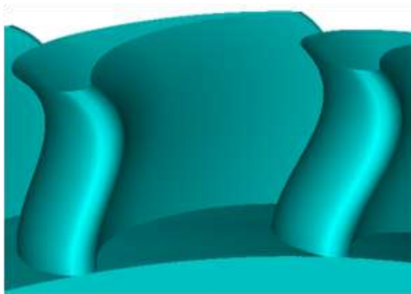
Figure 6.23 Optimal cascade obtained using method 1 for a/l = 0.23 .
