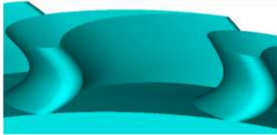
Figure 6.20 Optimal cascade obtained using method 1 for a/l = 0.44 .
