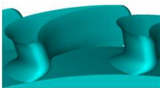
Figure 6.26 Optimal cascade obtained using method 2 for a/l = 0.44 .
