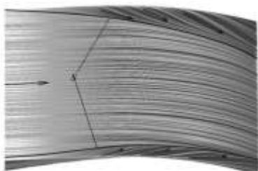
Figure 6.33 Stream lines on the suction side of the initial blade.
