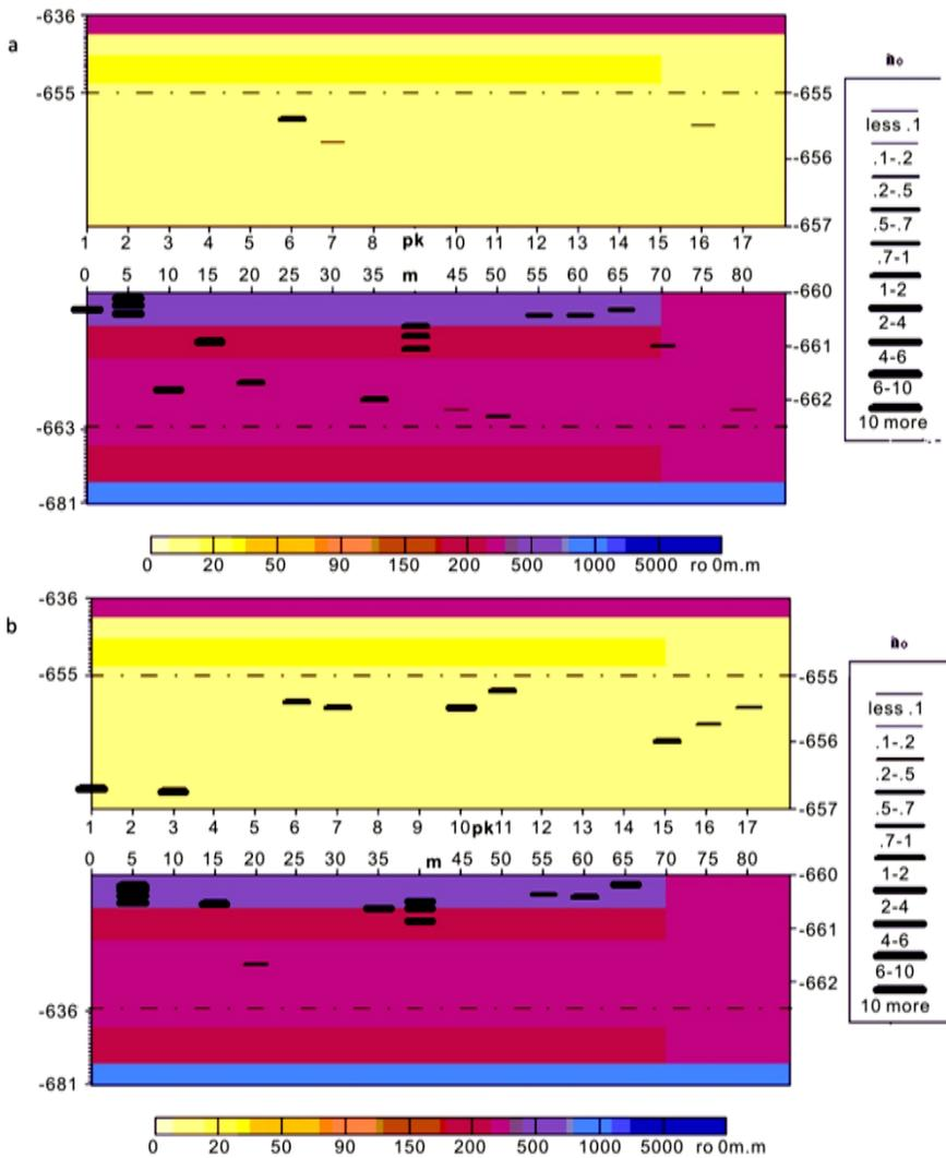
**Figure 3.** Geoelectrical sections along the profile in the Tashtagol mine for the depth 660m for two cycles of active electromagnetic monitoring during one week between the two cycles, the frequency was 10.15 kHz; a-data of the first cycle the 9-th of July 2010, b-data of the second cycle the 16-th of July 2010.
