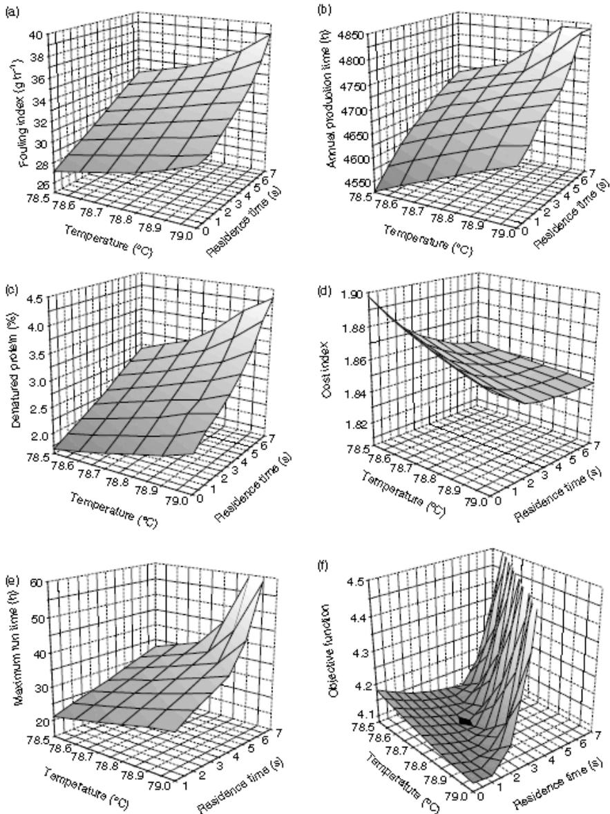
**Figure 2.4** Results of the optimization for different aspects of the objective function as a function of the control variables: (a) fouling index; (b) annual production; (c) protein denaturation; (d) cost index ( $\text{€ ton}^{-1}$ ); (e) maximum run time; (f) objective function evaluation. Source: Britz, J. T and Robinson, R. K. 2008.
